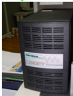
The LIBERTY 240/16: This is the base system, supports up to 16 sensors, each operating at up to 240 Hz.
