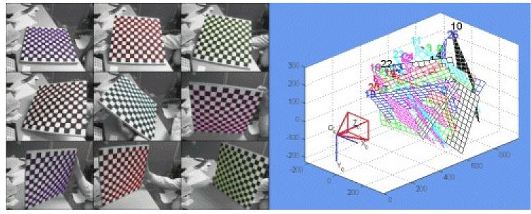
We used a matlab toolkit to calculate the intrinsic and extrinsic parameters of the cameras. Rotation and Translation matrixes between the cameras are also obtained.
