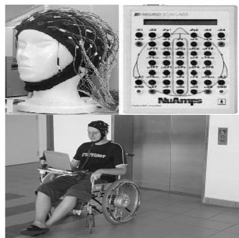
Fig. 2. Photographs of the acquisition devices and brain controlled wheelchair during experiments in a typical office environment. Note the compact portable system including signal amplifier, filter and acquisition device.
