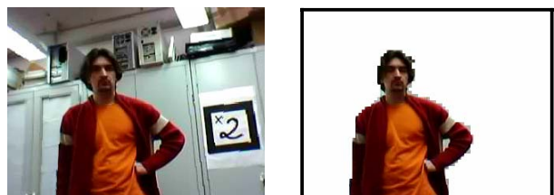
Fig 5 Object extraction in a complex environment.
