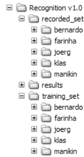
Figure 11: Directory structure of the database. The training_set folder contains a set of 20 face images per person. The recorded_set folder contains 250 images per person and along this report is referred as test set. In the results folder we store some important information collected during run time
